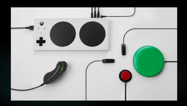
Designed primarily to meet the needs of gamers with limited mobility, the Xbox Adaptive Controller is a unified hub for devices that helps make gaming more accessible.
