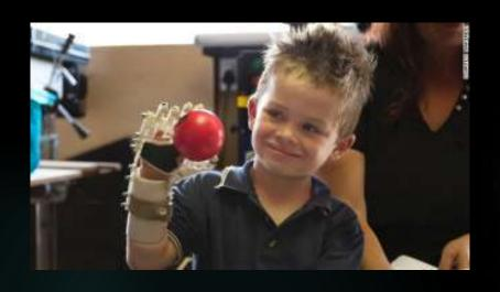
"Officially launched in January 2012, Robohand creates affordable mechanical prosthetics through the use of 3D printers. Not only that, but it has made its designs open source, so that anyone with access to such printers can print out fingers, hands, and now arms as well."
