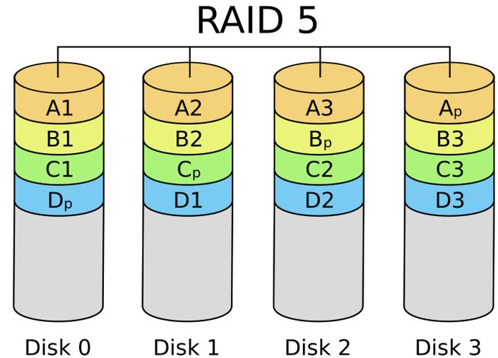
Striping + 1 parity disk: adds performance and reliability at lower storage cost
