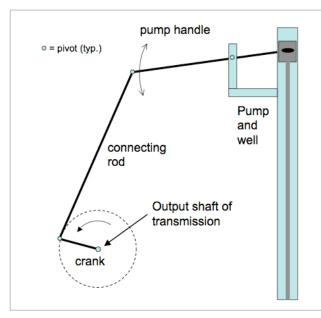
(like you sometimes see at campgrounds in the US). Your project involves setting up an engine and transmission to power a rockercrank linkage to pump the handle up and down. After considering various possibilities, you decide on a small steam engine, mainly because it can burn almost any liquid fuel from biodiesel to ethanol. The steam could even be generated partly by a thermal solar collector. Also, with care, it can have efficiency comparable to an internal combustion engines.<sup>1</sup>
