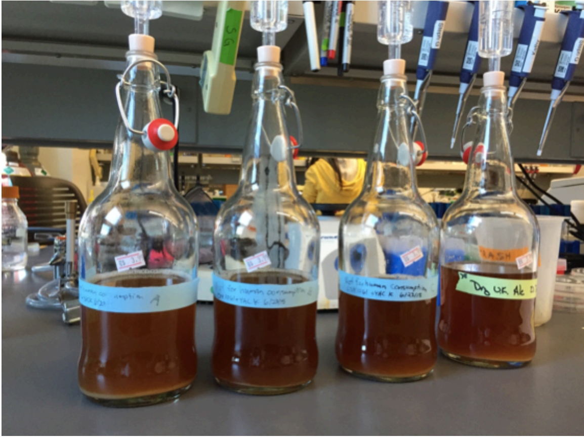
Figure 2. Small volume ‘home-brew’-style fermentation of yeast engineered to produce thebaine (three left bottles) or adapted to produce an English ale (right bottle, positive fermentation control).
